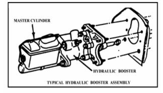
3. Condition of hydraulic booster power brake system. Inspect system for fluid level and leaks.
