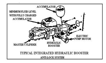
5. Condition of integrated hydraulic booster/anti-lock system with electronic pump. With the system fully charged, inspect system for fluid level and leaks.
