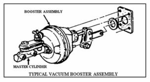
7. Condition of vacuum booster power brake system. Reject vehicle if there are collapsed, cracked, broken, badly chafed or improperly supported hoses and tubes, loose or broken hose clamps.
