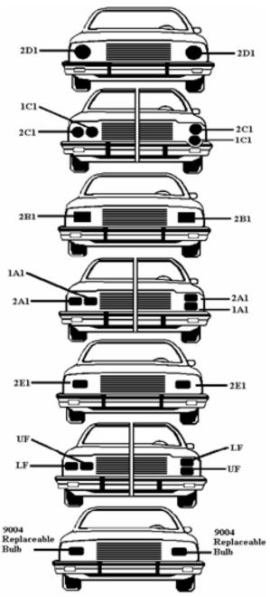
Locations of Type 1, Type2, LF/UF, and Replaceable Bulb Headlamps
